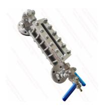
Transparent level gauges are always fitted with two plate transparent glasses between which the fluid is contained. The fluid level is indicated as the result of the different transparency of the two media and in some cases (for water steam), by conveying upwards on to the surface of separation (between liquid and gaseous substances) a source of light located at the back of the gauge, the rays of which are totally reflected down to the observer.
